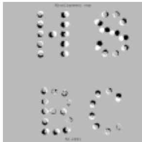
Figure 5. Misalignment map of holes in two HS/BC patterns.
